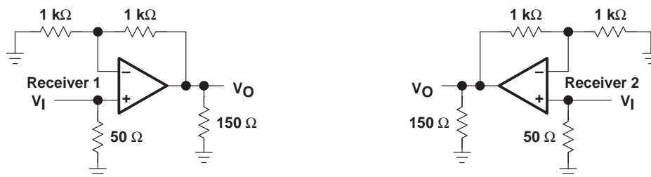
Figure 2. Receiver Input-to-Output Crosstalk Test Circuit
